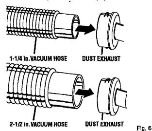
NOTE: A standard 1-1/4 in. vacuum hose connection fits inside the smaller diameter hole inside the dust exhaust, while a standard 2-1/2 in. vacuum hose connection fits inside the larger hole of the dust exhaust.
